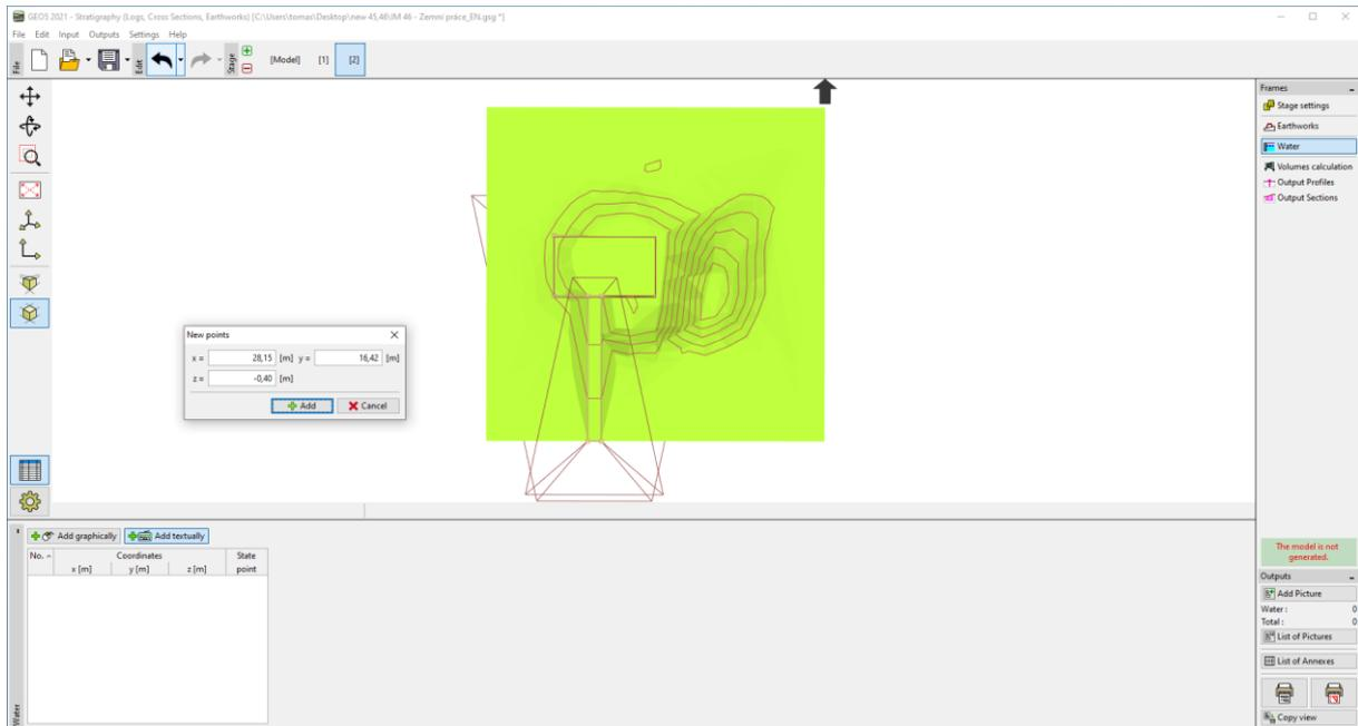
In the „Volumes Calculation“ frame, we will calculate the volume of the excavated and filled soil.
