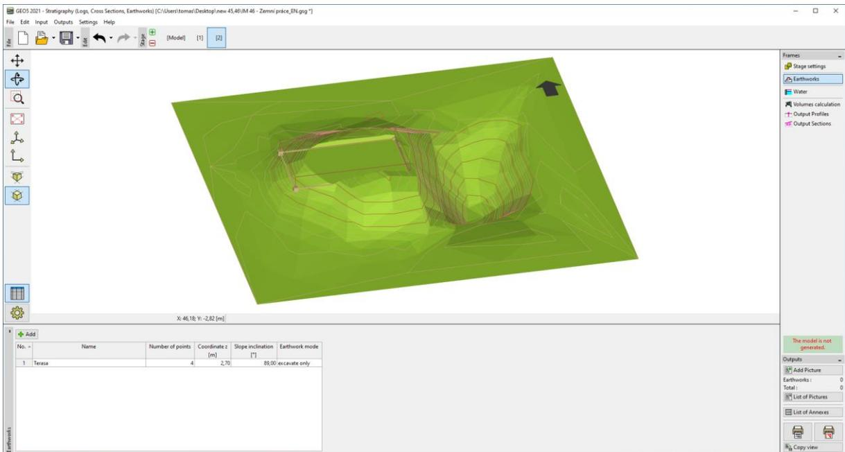
We will enter another earthwork, this time representing the access ramp. For simplicity, we will choose a rectangle with coordinates: [28;35], [50;35], [50;33], [28;33]. The height of the adjustment is a variable this time – at the top, the height is 2.7m, down it is 0.0m and a slope of 30 degrees. We will be adding and removing the soil this time – therefore, we will choose the mode: „Fill and excavate“ mode.
