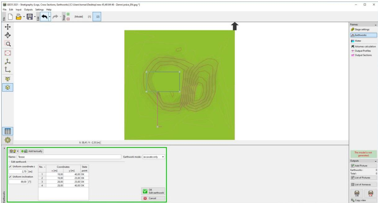
The created construction will be generated after entering. The outline of the earthwork that cut the terrain is shown in red.
