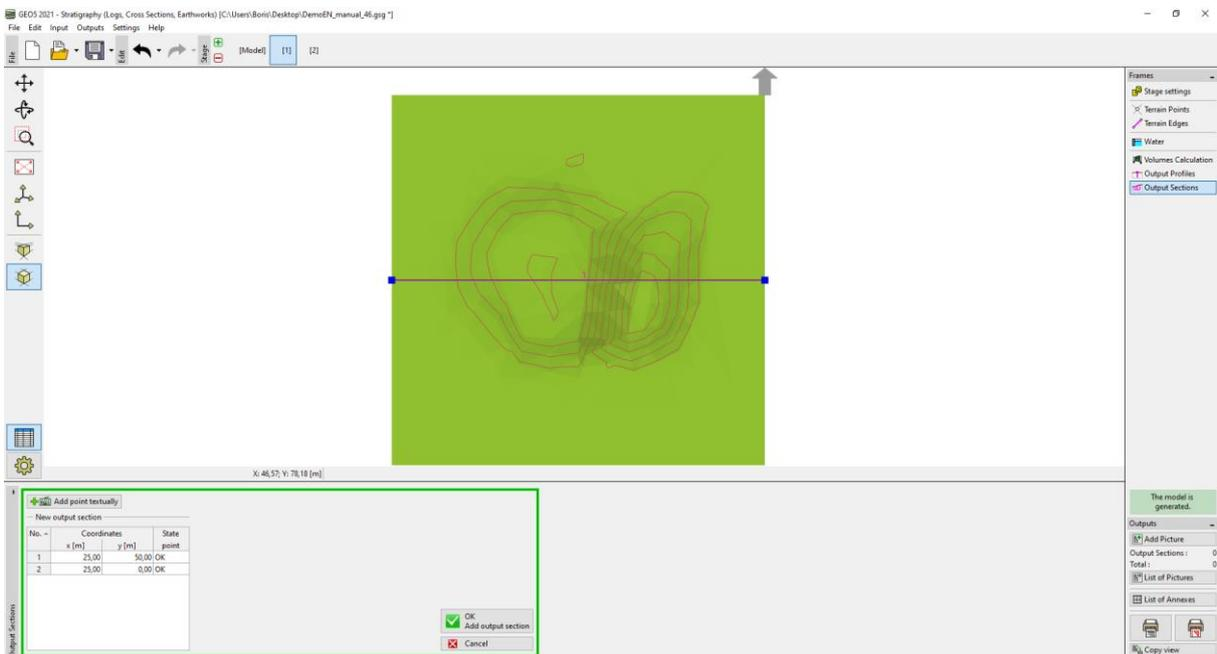
We will name and save the created cross-section. The red line in the section shows the terrain from the previous construction phase resp. the terrain of the original model.
