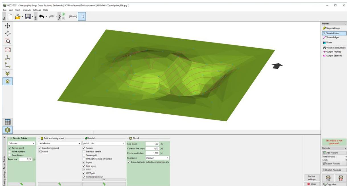
We will switch to the „Volumes Calculation“ frame. We will input a new soil, that forms the created embankment and generate the model. In the frame, we have the calculated volumes of embankments and excavated soils.
