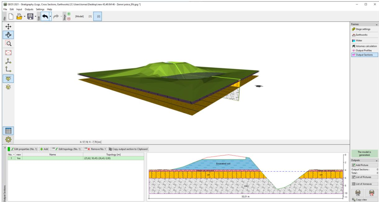
Then we will go to the “Slope Stability” program (menu item „Edit“ „Paste data“), where we will insert the cross-section. After entering the soil parameters, surcharge, and calculation parameters, we can then analyse the construction.
